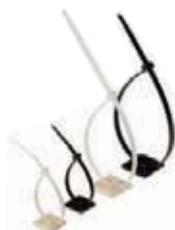
CB cable ties provide fixings for cables and markers for special requirements. They are especially suitable for fixing CLI M, SFX, WKM and WKS cable markers. The material consists of unbreakable polyamide PA 6.6 with UL94 flammability rating V2.
