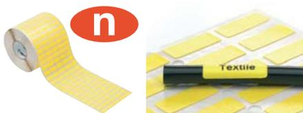
Textile labels are made of very flexible cotton fabric. The delivery form in rolls is made for using thermal transfer printers. Thus a ticker adhesive layer is possible as with labels on A4 sheets. Both, the flexible material and the ticker adhesive layer, offers a better adhesive power and allows the use for angled or round object like cables or tubes.
